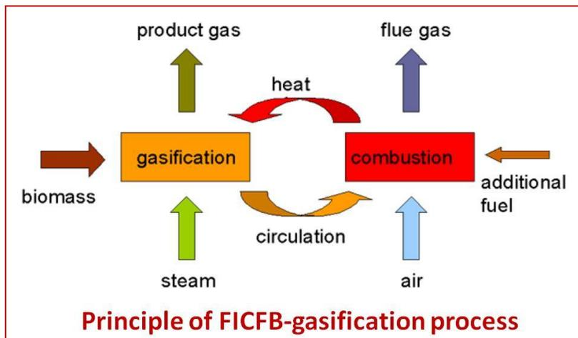
gasified with steam and releases a mixture of combustible gases, such as CO<sub>2</sub>, CO, H<sub>2</sub>, etc. and water vapours. A chute connects the gasification section with the combustion section and combustion reactor operates as a circulating fluidised bed. Bed material from the gasification chamber together with any non-gasified carbon is transported through this
